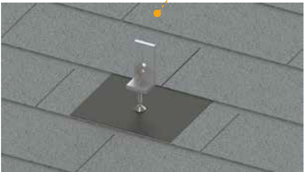
Fix the L-shaped leg and the waterproof board to the beam with bolts.
